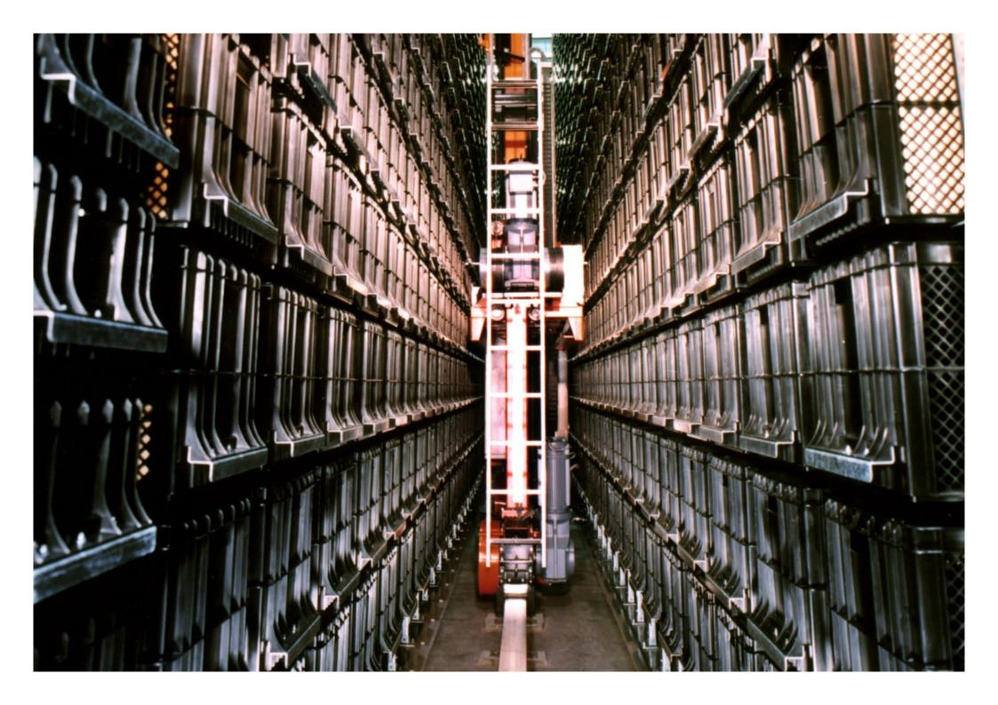
"Dexion was contracted to design and implement an automated storage and retrieval system capable of processing and shipping up to 19 million items a day."
