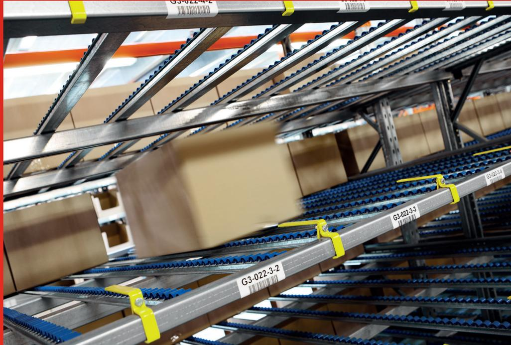
Lead in guides ensure pick positions are clearly identified and maintained when goods are being replenished.
