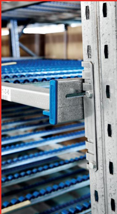
Beds are mounted directly to uprights eliminating the need for additional beams.
