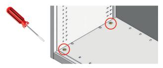
Each levelling foot allows for a maximum of 20mm of adjustment, the cabinet must not be adjusted further than 20mm from the ground at any point.
