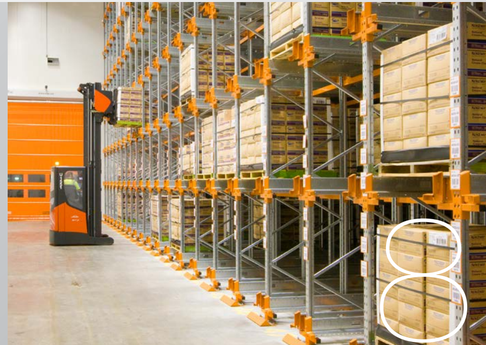
The shuttle unit deposits and retrieves pallets within the high density core of the Auto Shuttle system.
