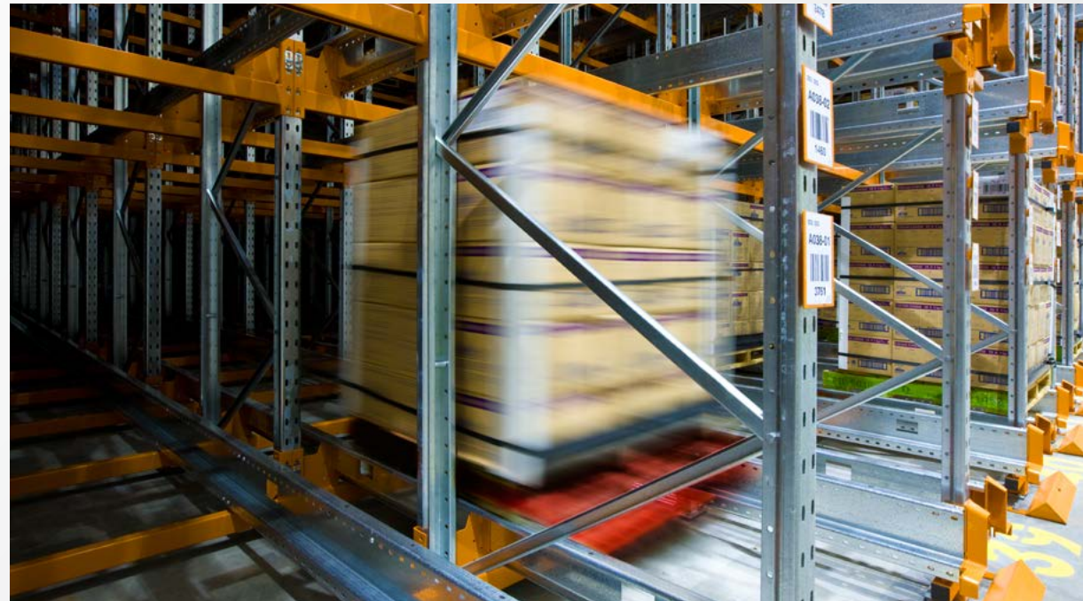
The shuttle unit deposits and retrieves pallets within the high density core of the Auto Shuttle system.
